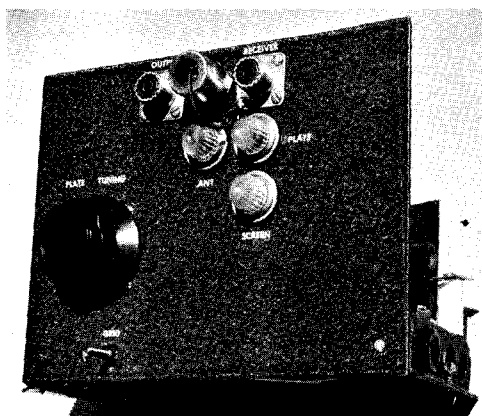
Figure 13 MIDGET LINEAR AMPLIFIER FOR MOBILE SIDEBAND OPERATION FEATURES WATER COOLED 4W-300B TETRODE TUBES
