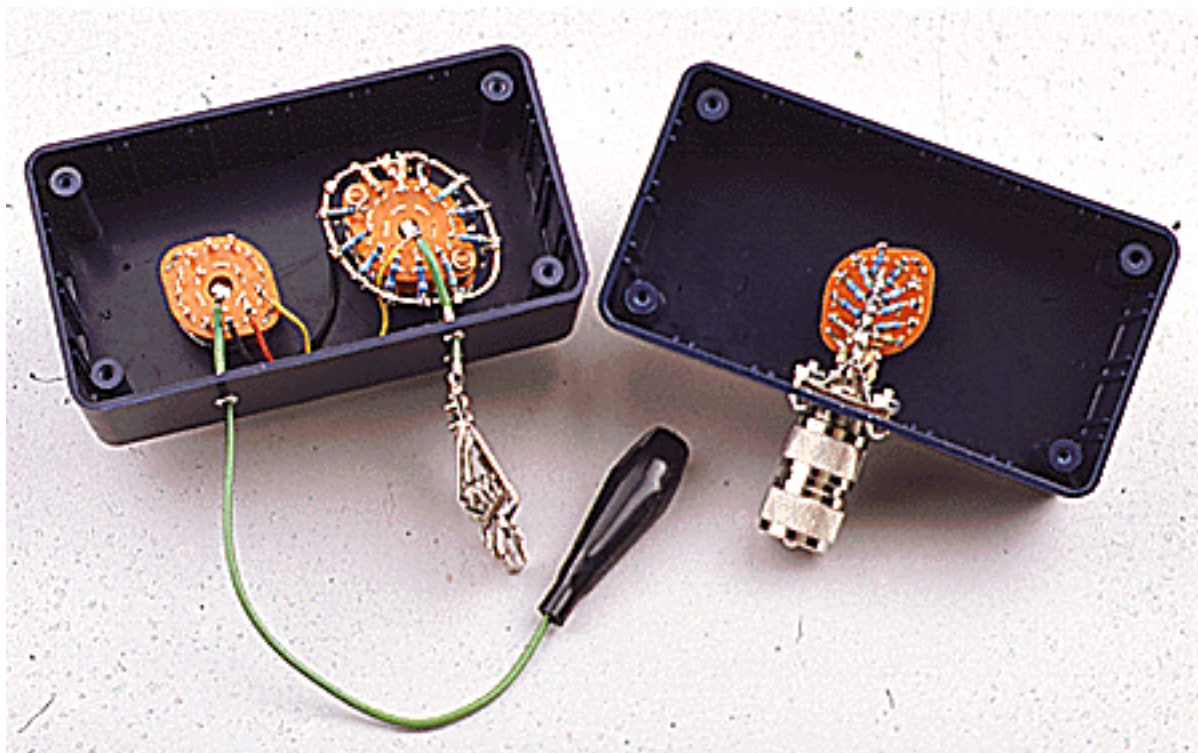
Figure 3—Photo showing inside of Geometric Resistance Boxes. The resistor leads and connections to the load switches
